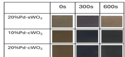
Fig. 4. Color change in WO 3 sensors for sensitive hydrogen detection. 300 s of H 2 /N 2 exposure followed by 300 s of air exposure
