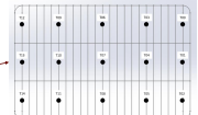
Fig 2 - Schematic representation of thermocouple placement across the oven rack to monitor temperature distribution
